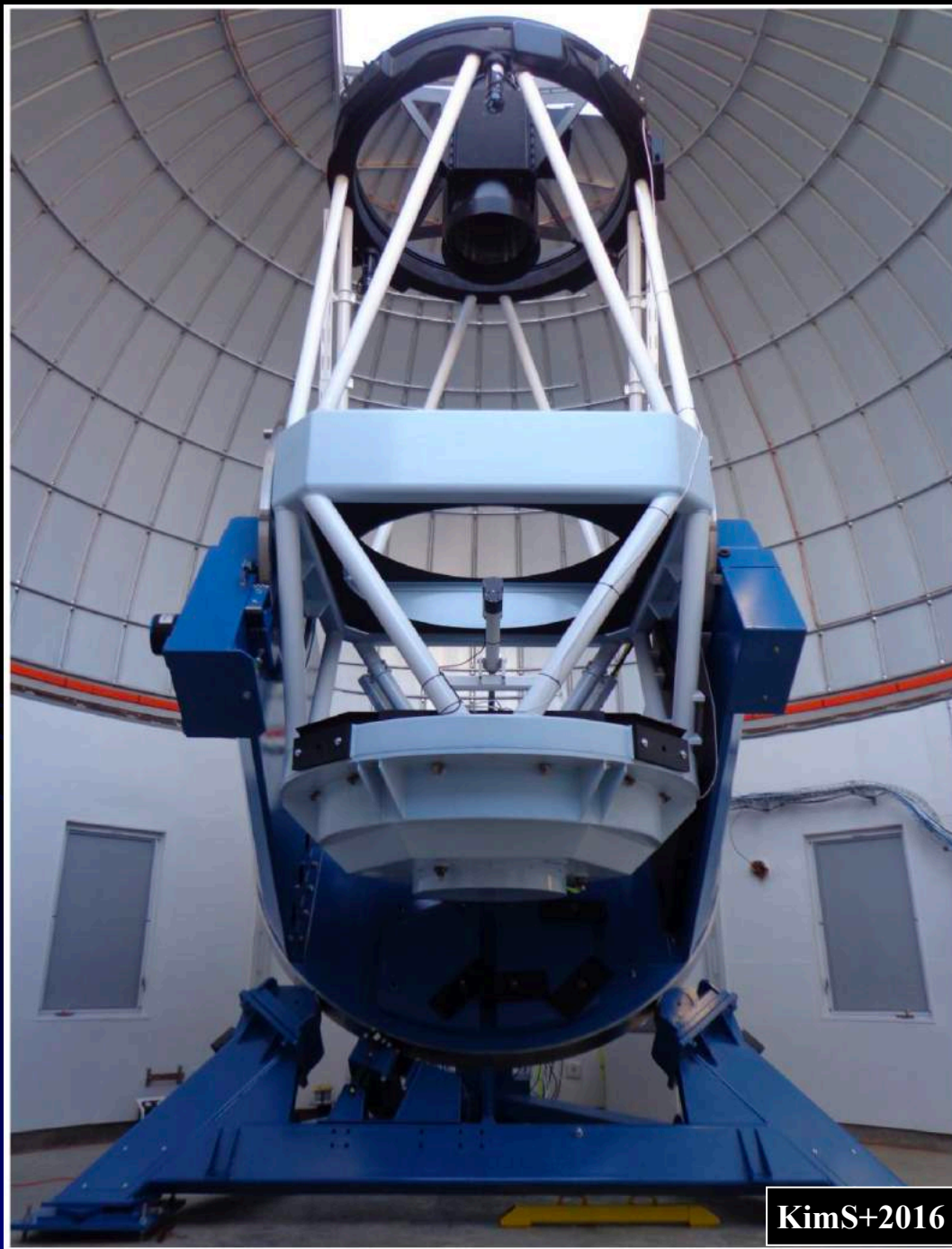
Figure 4. (Top) The camera's focal plane assembly mounted with four mosaic science CCDs and four small guide CCDs. (Bottom) The camera attached to the KMTNet telescope at CTIO. The head electronic box is mounted on the telescope top ring, shown at the left.
