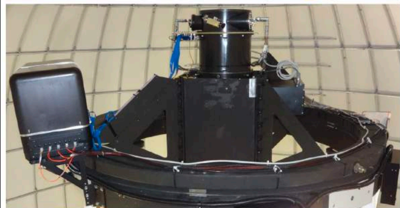
Figure 4. (Top) The camera's focal plane assembly mounted with four mosaic science CCDs and four small guide CCDs. (Bottom) The camera attached to the KMTNet telescope at CTIO. The head electronic box is mounted on the telescope top ring, shown at the left.
