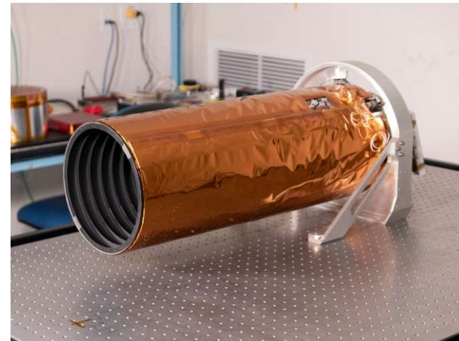
ShadowCam (118x28 \varnothing cm, 8.8 kg)
