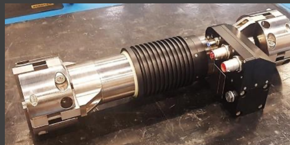
Prototype hexapod positioner actuator
