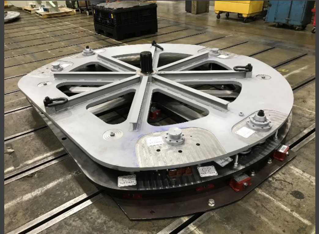
Mirror cell positioner alignment & repeatability test
