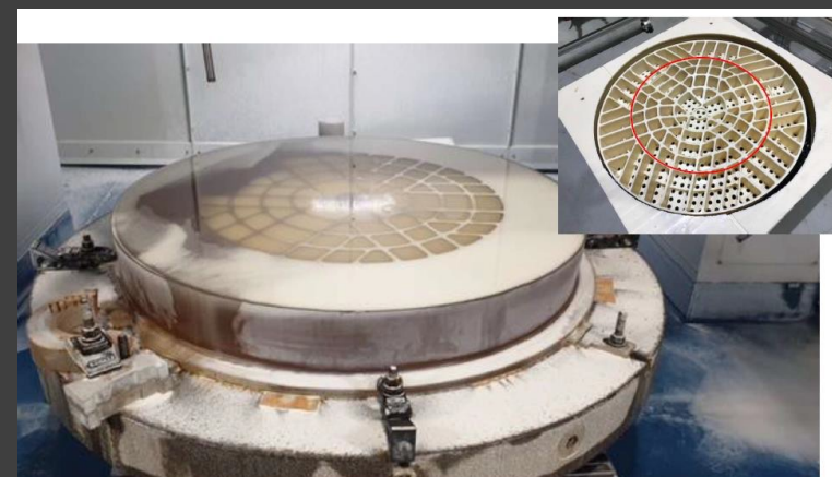
ZeroDur ASM reference body being machined
